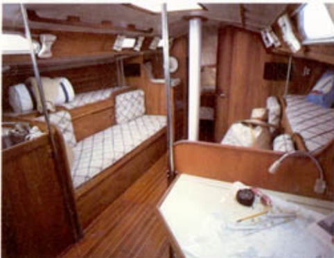
Classic yacht layout (2 settees with a pilot), classic yacht finish (teak bulkheads and trim), classic satin varnished teak and holly cabin sole.
