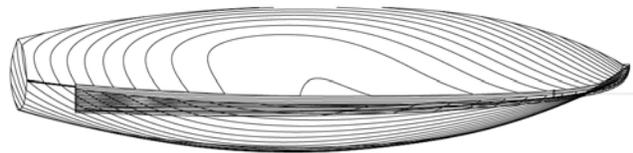
Figure 28 – Waterlines of hull BL049 at 20° heel
