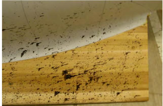
Figure 41 – Oil streak flow visualization; Keel C
