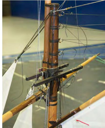
Figure 47 – Detail of the standing rig.
