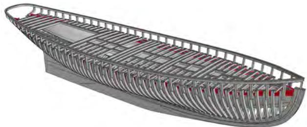
Figure 33 – *Rhino* model of primary hull structure
