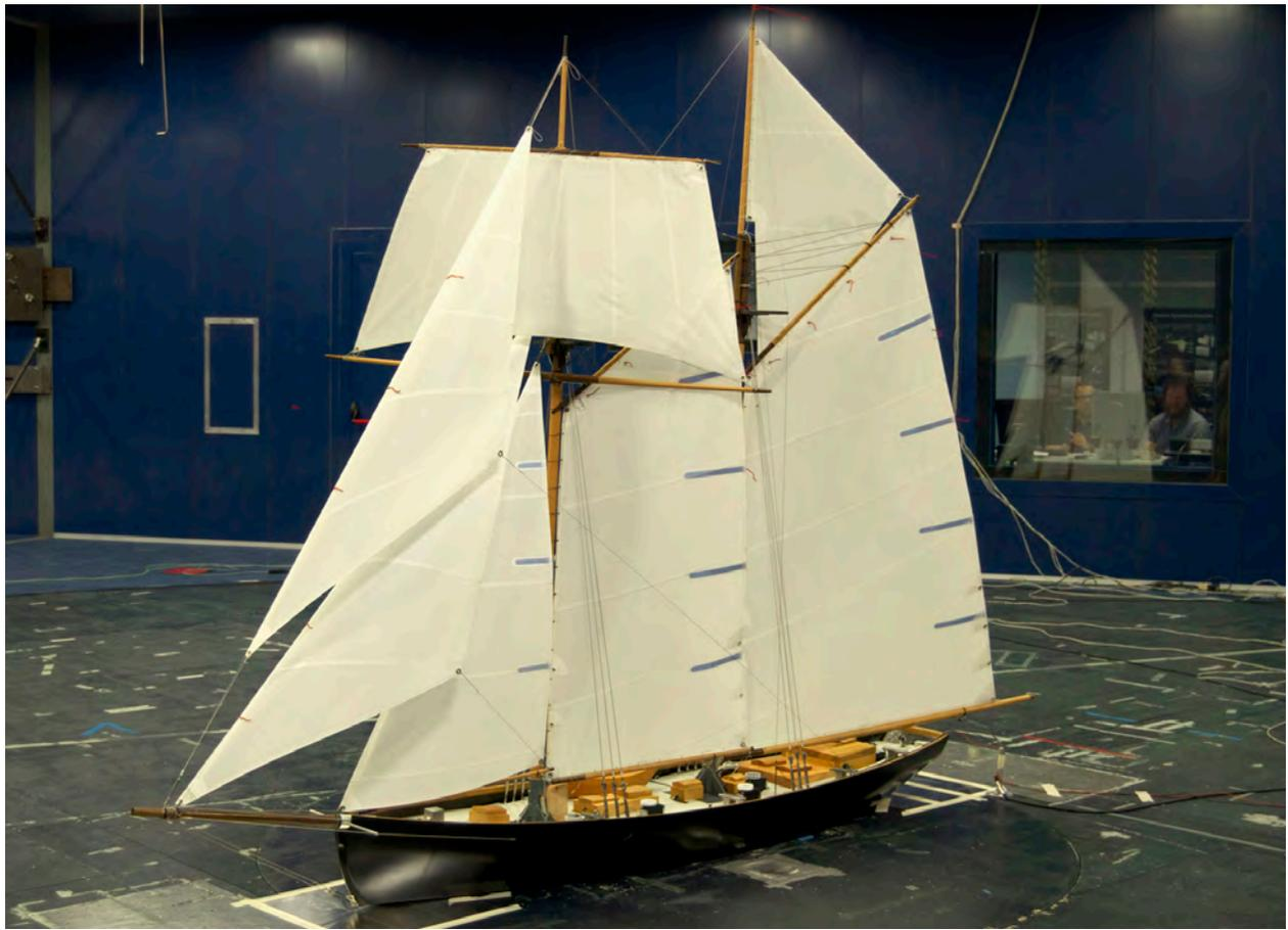
1:15 scale model of SALTS' new schooner in the Politecnico di Milano boundary layer wind tunnel
