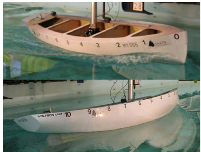
Figure 38 – 12 knots ( $F_n = 0.36$ ) 15° heel
