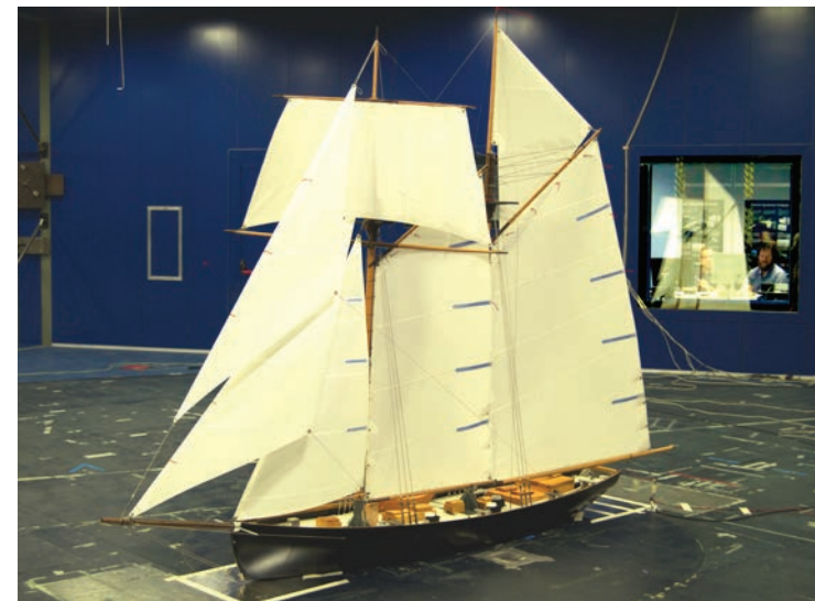
Wind Tunnel Testing of a Rigging Model
