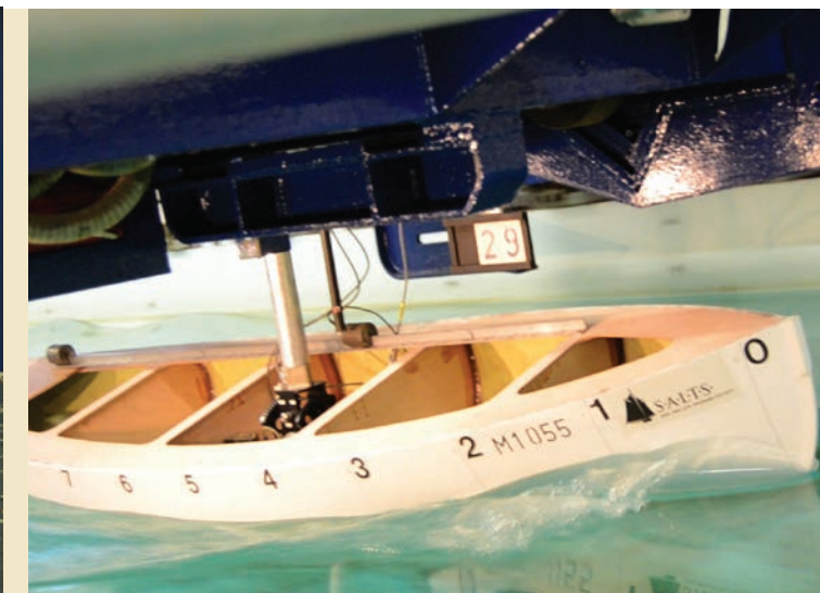
Towing Tank Testing of a Hull Model
